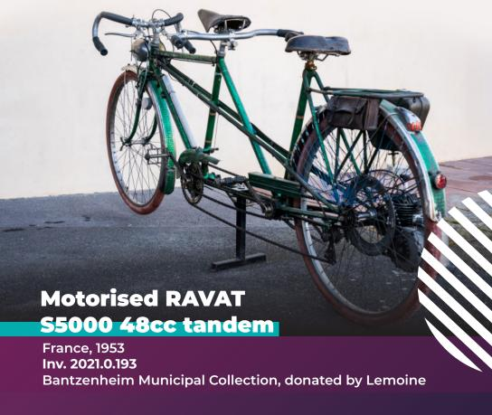
The Ravat tandem is an oddity and there aren't many of them around. Ravat only made a few because the engine on the side of the rear wheel caused significant imbalance and it was dangerous to ride.
